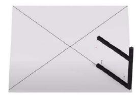
Align the legs to cover the corner lines and insert the screws.
