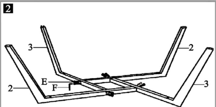
Do not fully tighten the bolts at this stage
