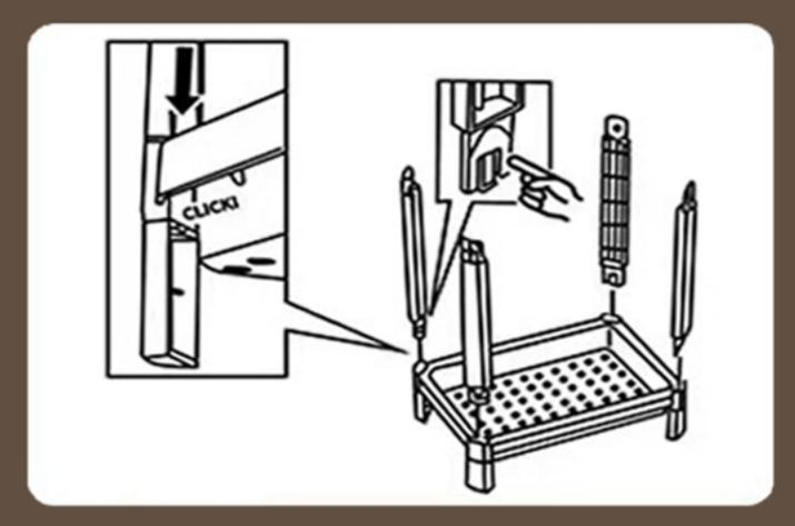
2. Insert the four stand columns into the upper grooves of the basket;
