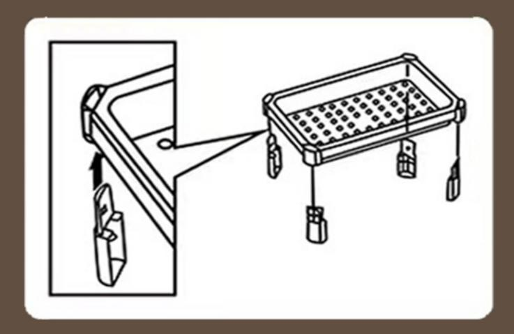
1. Insert the bottom foot into the groove at the bottom of a basket;
